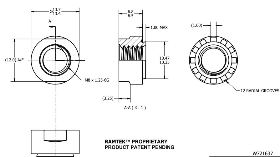
1. MATERIAL: ISO 898-2 (10) 2. HARDNESS: HRc 35 - 39 3. PROOF LOAD: 38.1 kN
